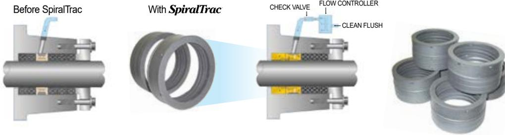
Reduced Flush · For use with packing only · No pump upgrade required
